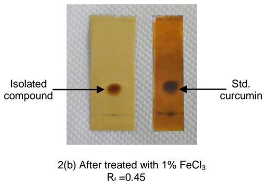
Fig. 2. TLC chromatograms of isolated compound and standard curcumin
