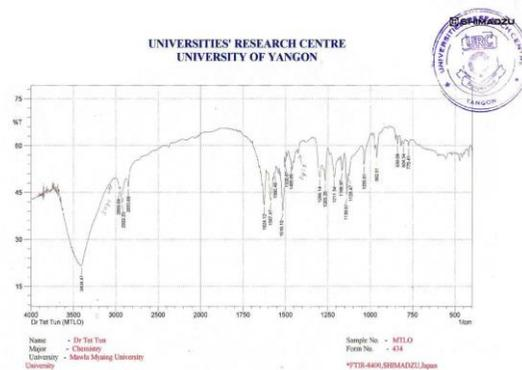
Fig. 4. FTIR spectrum of isolated curcumin
